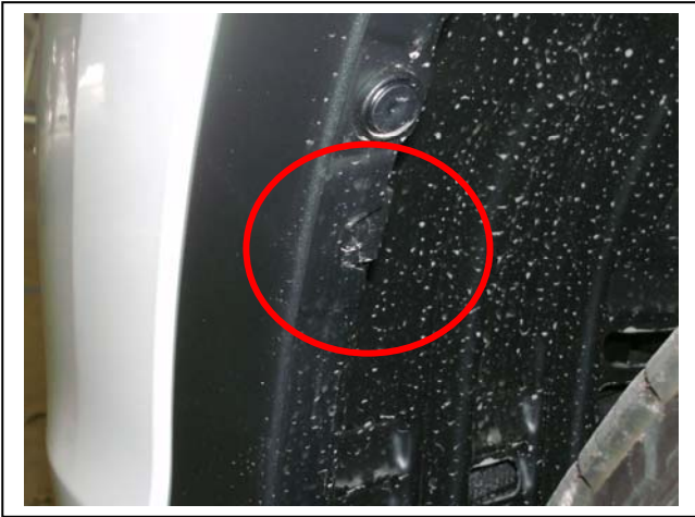
Figure 1: Placement of hidden plastic clip. Turn centre ½ turn and remove.
